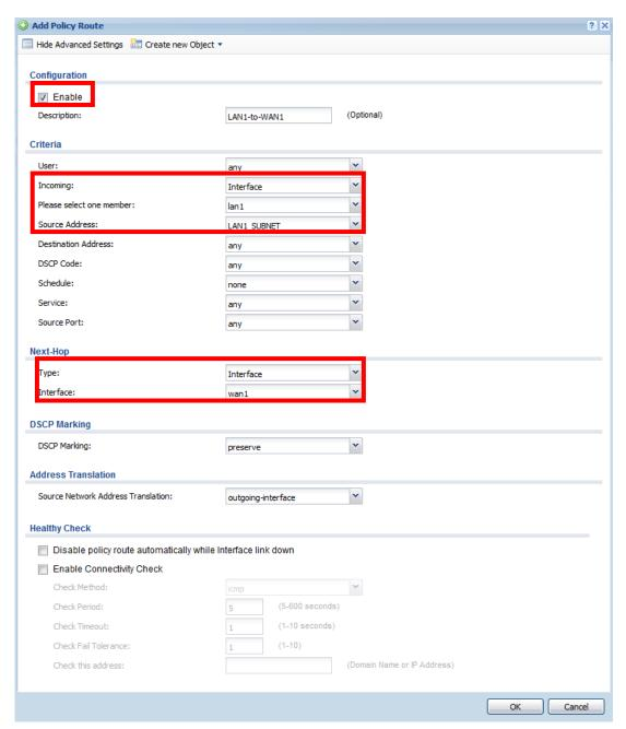
Note: Check the "Disable policy route automatically while Interface link down" to have the route disable automatically if WAN\* is down and use the live connection for backup.
