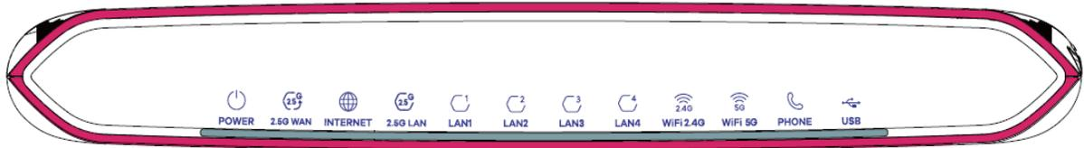
None of the LEDs are on if the Zyxel Device is not receiving power.
