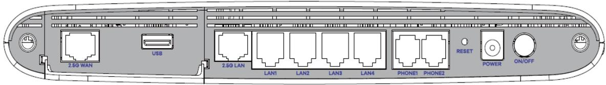
Figure 23 PX7501-B0 Bottom Panel
