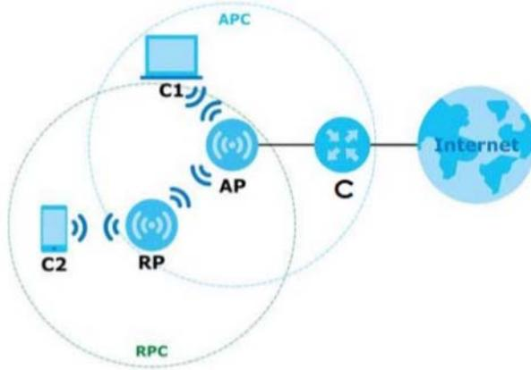
A controller can automatically configure WiFi settings on extenders in the network as well as optimize bandwidth usage. The controller optimizes bandwidth usage by directing wireless clients to an extender (AP steering) or 2.4G or 5G band (band steering) that is less busy.
