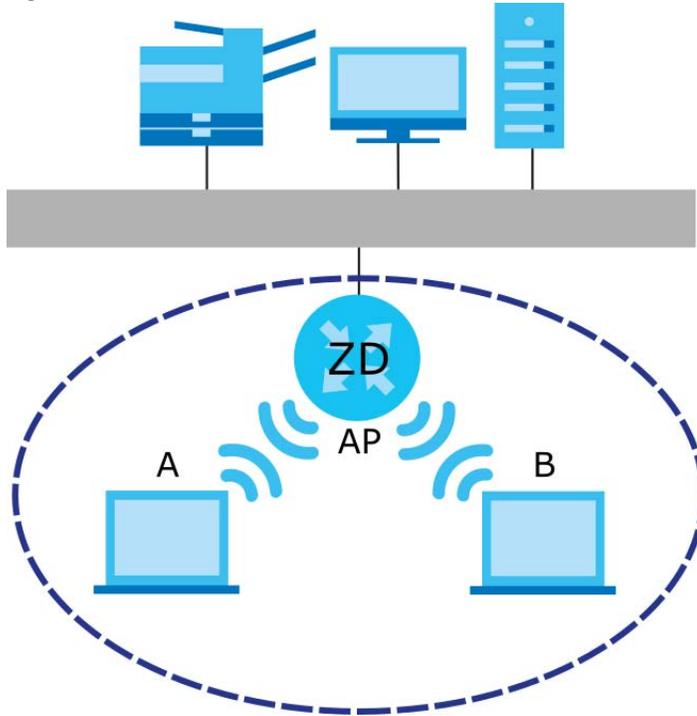
The WiFi network is the part in the blue circle. In this WiFi network, devices **A** and **B** use the access point (**AP**) to interact with the other devices (such as the printer) or with the Internet. Your Zyxel Device is the AP.
