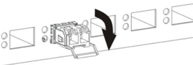
**Figure 29** Transceiver Removal Example
