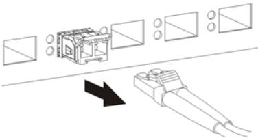
**Figure 28** Opening the Transceiver's Latch Example
