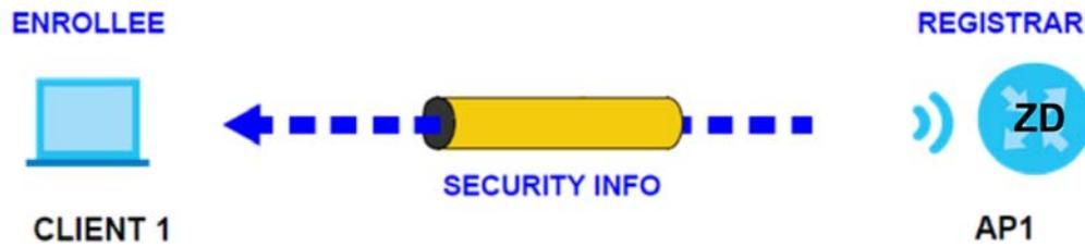
In step 2, you add another WiFi client to the network. You know that **Client 1** supports registrar mode, but it is better to use **AP1** for the WPS handshake with the new client since you must connect to the access point anyway in order to use the network. In this case, **AP1** must be the registrar, since it is configured (it already has security information for the network). **AP1** supplies the existing security information to **Client 2**.
